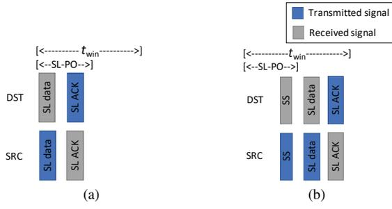
Fig. 3. SCUBA synchronization when (a) the SRC is in fine sync with the DST, and (b) when the SRC is not.
