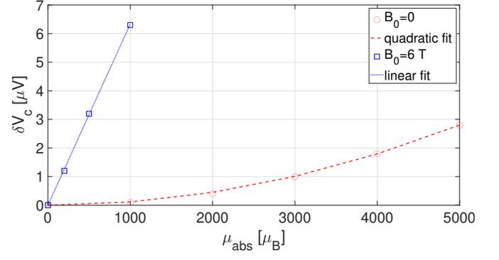
FIG. 11. The impact of a magnetic dipole moment  $\mu_{abs}$  on the critical voltage  $\delta V_c$  at  $T = 0$  in the presence/absence of a background uniform magnetic field  $B_0 = 6$  T. Device parameters:  $N = 51$ ,  $\Gamma = 1.7$  meV,  $U = -50$  meV.
