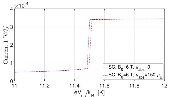
FIG. 12. The I-V characteristics of the device at  $T = 0$  in the presence of a background uniform magnetic field  $B_0 = 6 \text{ T}$  and without/with a magnetic dipole moment  $\mu_{abs} = 150 \times \mu_B$ . Device parameters:  $N = 51$ ,  $\Gamma = 1.7 \text{ meV}$ ,  $U = -50 \text{ meV}$ .
