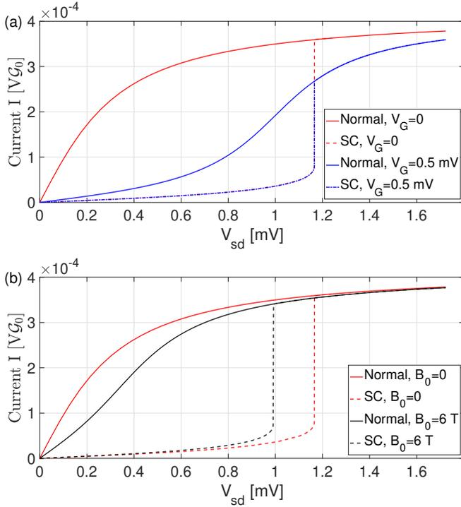
FIG. 10. Bias voltage dependence of the current at  $T = 0$  for two different types of perturbations: a) Uniform gating potential  $V_G = 0.5$  mV b) Uniform magnetic field  $B_0 = 6$  T. Device parameters:  $N = 51$ ,  $\Gamma = 1.7$  meV,  $U = -50$  meV.
