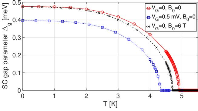
FIG. 9. Temperature dependence of the SC gap parameter  $\Delta_g$  in the absence/presence of several external perturbations such as a uniform gating potential  $V_G = 0.5$  mV or a uniform magnetic field  $B_0 = 6$  T. Device parameters:  $N = 51$ ,  $\Gamma = 1.7$  meV,  $U = -50$  meV.
