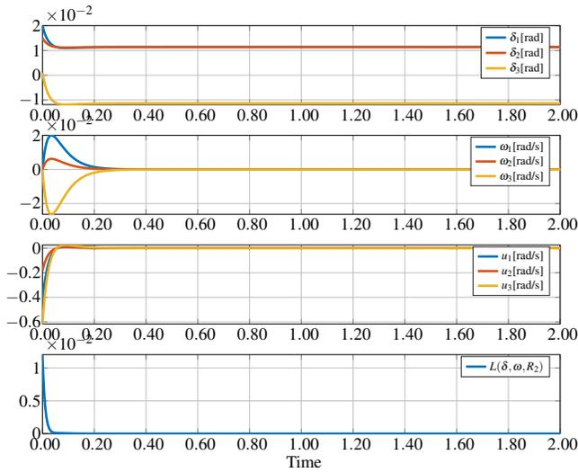
Fig. 3. Simulations for  $w = 0$  of angle differences, frequencies, inputs and the cost function after closing the loop with the optimal control (22) for  $R_2 = 0.1 \cdot R_1$ . The error decay transients of the angles and frequencies improve significantly with more control effort (compared to Figure 2). The nominal cost function  $L(\delta, \omega, R_2)$  decays towards a nearby zero value.
