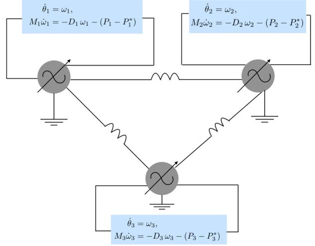
Fig. 1. Three inverter system with dynamics given in (18), where  $P_i = \sum_{j \in \mathcal{N}_i} b_{ij} \sin(\theta_{ij})$  and  $P_i^* = \sum_{j \in \mathcal{N}_i} b_{ij} \sin(\theta_{ij}^*)$  for  $i = 1, 2, 3$ .
