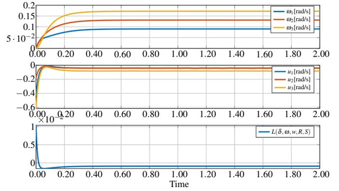
Fig. 4. Simulations of the frequencies, input and cost function of the three-inverter system for constant non-zero disturbance  $w$  in closed-loop with (22) for  $R = 0.01 \cdot I_3$ ,  $S = I_3$  and  $\xi = 2.8 > \frac{1}{4D}$ . The frequencies remain bounded and the cost function  $L(\delta, \omega, w, R, S)$  in (1) takes negative values with a randomly generated disturbance  $w \neq w^*(x)$ .
