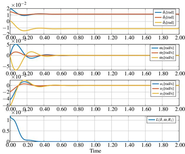
Fig. 2. Simulations for  $w = 0$  of angle differences, frequencies, inputs and the cost function of the three inverter system described in Figure 1 for  $w = 0$  after closing the loop with the optimal control (22) with  $R_1 = 0.1 \cdot I_3$ . The angles are stabilized at the specified steady state and the frequencies synchronize and decay towards zero. The cost function  $L(\delta, \omega, R_1)$  strictly decreases towards a nearby zero value.
