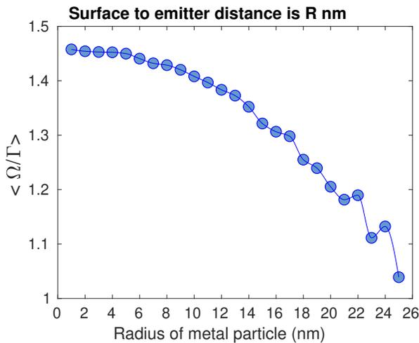
FIG. A2. Polarization averaged coupling strengths of a single emitter and a gold nanoparticle as determined by the Markovian model, which can be used for one-loop corrections.
