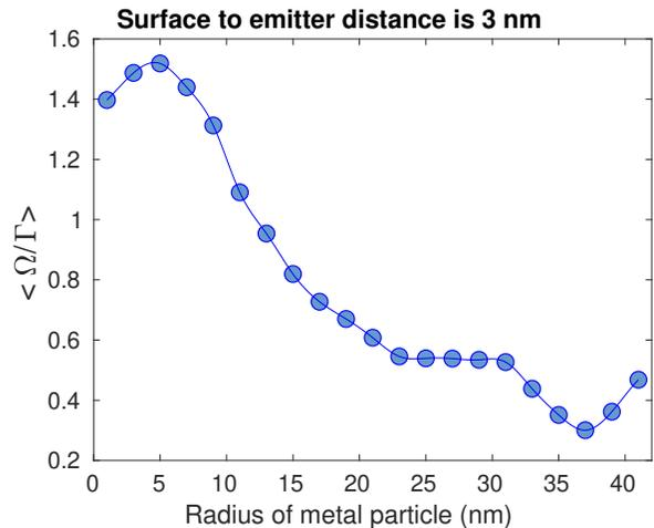
FIG. A1. Polarization averaged coupling strengths of a single emitter and a gold nanoparticle as determined by the Markovian model, which can be used for one-loop corrections.
