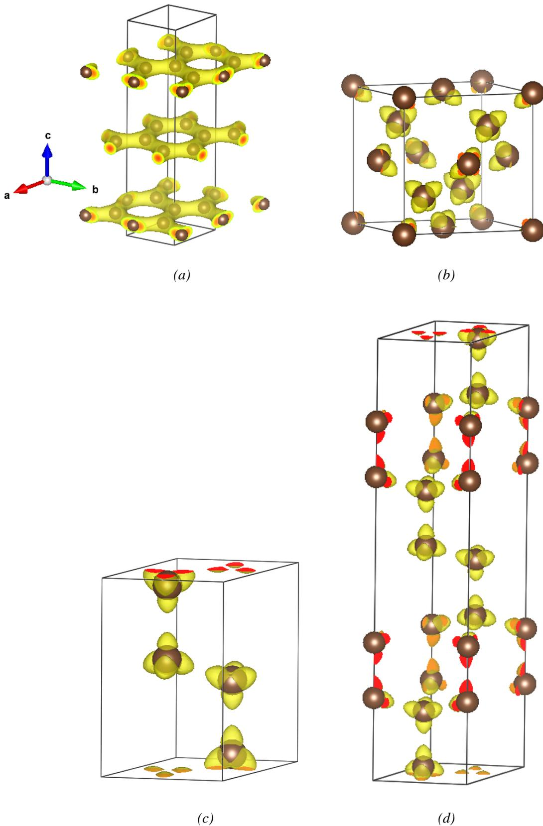
Figure 2. Charge density.  $C(sp^2)$ -like rings in (a) *rh-C<sub>2</sub> 3R* graphite; and  $C(sp^3)$ -like tetrahedra in: (b) *c-C<sub>8</sub>* diamond; (c) *h-C<sub>4</sub>* lonsdaleite and (d) *rh-C<sub>4</sub> (h-C<sub>12</sub>)* rhombohedral carbon. Brown spheres represent the carbon atoms.
