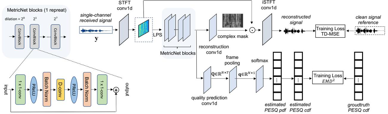
Figure 1: The overall MetricNet model architecture and the convolutional structure of MetricNet blocks. Each block (ConvBlock) consists of a  $1 \times 1$ -conv layer, a depth-wise separable convolution layer ( $D$ -conv), with PReLU activation function and normalization added between each two convolution layers. The residual connection is added in each block.
