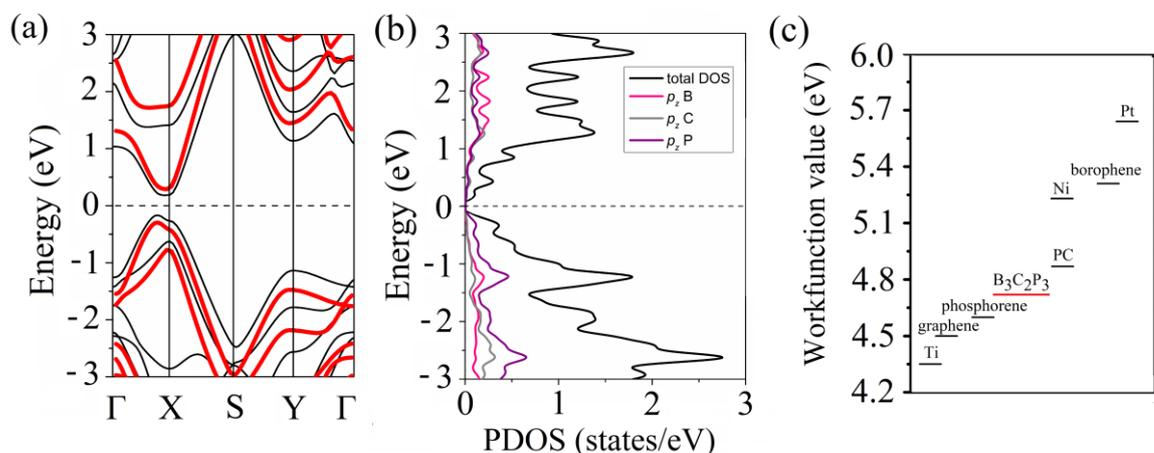
**Figure 2.** (a) Band structure of 2D  $B_3C_2P_3$ . The black and red lines show the band structure calculated by the PBE and HSE approaches. (b) PDOS of 2D  $B_3C_2P_3$  (calculated by the PBE). (c) Comparison of the workfunction of  $B_3C_2P_3$  with those of common 2D materials and bulk metals.
