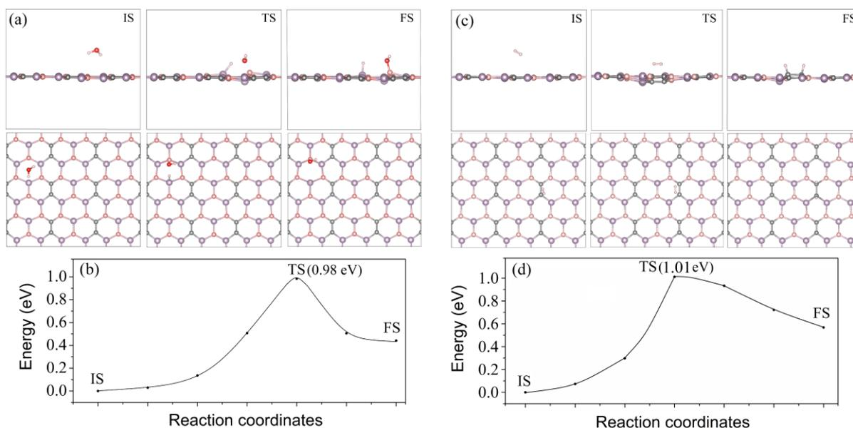
**Figure 3.** The atomic configurations and energy profiles of the reaction pathway from the physisorbed (IS) to the chemisorbed (FS) state in the dissociation process of (a) and (b)  $\text{H}_2\text{O}$  and (c) and (d)  $\text{H}_2$  molecules on 2D  $\text{B}_3\text{C}_2\text{P}_3$ .
