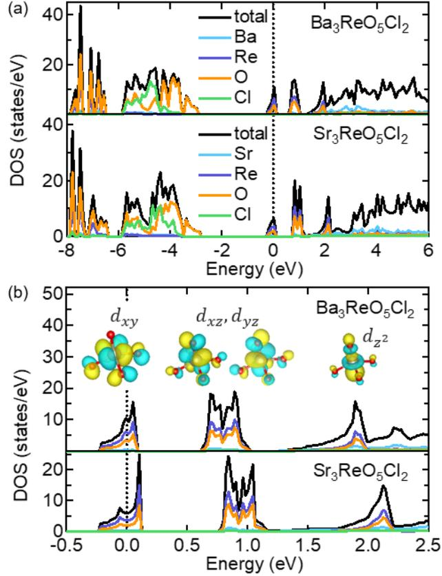
Figure 6. (a) Density of states (DOS) for BROc and SROc obtained by first-principles calculations based on the density functional theory using the program package Quantum ESPRESSO. The Fermi energy ( $E_F$ , vertical dotted line) is set at zero. Partial DOSs for Ba or Sr (light blue), Re (purple), O (orange), and Cl (light green) are distinguished by color lines. (b) DOS near  $E_F$  and the corresponding 5d orbitals of Re mixed with the 2p orbitals
