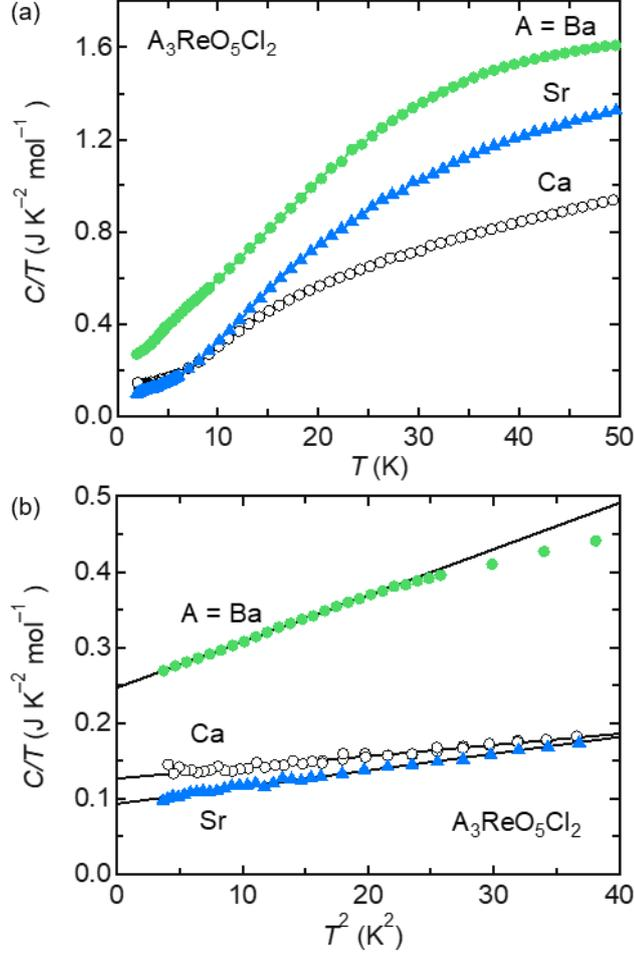
Figure 5. Heat capacity divided by temperature  $C/T$  as a function of  $T$  below 50 K (a) and as a function of  $T^2$  below 6 K for BROc (green filled circle), SROc (blue filled triangle), and CROc (open black circle). The black lines in (b) represent fittings to the equation  $C/T = \alpha + \beta T^2$ .
