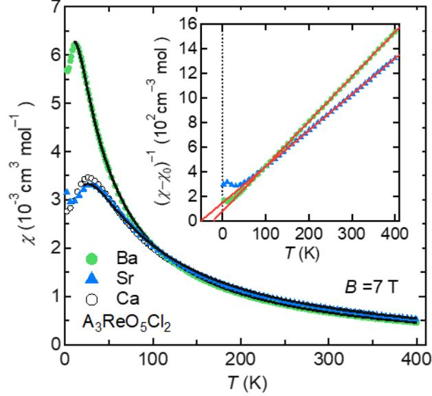
Figure 4. Temperature dependences of magnetic susceptibilities of the powder samples of BROc (green filled circle) and SROc (blue filled triangle) measured upon cooling in a magnetic field of 7 T. The data of CROc (black open circle) is also shown. The curve on each dataset represents a fit to the ATL model. The inset shows the inverses of the magnetic susceptibilities with Curie–Weiss fittings (red lines).
