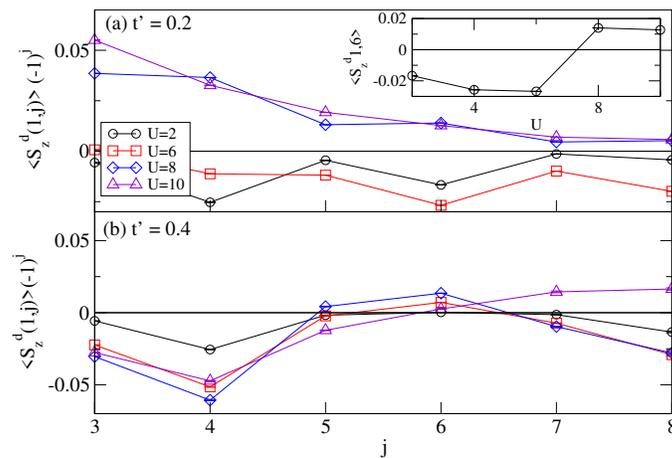
**Figure 2.** Dimer spin-spin correlations  $\langle S_z^d(1,j) \rangle$  for a  $16 \times 4$  lattice between the first dimer on chain 1 and dimer  $j$  on chain 2, multiplied by  $(-1)^j$ , the expected sign for Néel AFM. (a)  $t' = 0.2$ . The inset shows the  $U$  dependence of a single spin-spin correlation at long distance. Néel AFM order is present at  $t'$  for  $U \gtrsim 8$ . (b)  $t' = 0.4$ . Here we find no AFM order.
