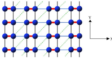
**Figure 1.** The dimer lattice we consider. Thick lines are the intra-dimer hopping  $t_d$ , thin lines are the inter-dimer hopping  $t$ , and dashed lines are the frustrating bond  $t'$ . Boundary conditions in our DMRG calculations are open in  $x$  and periodic in  $y$ .
