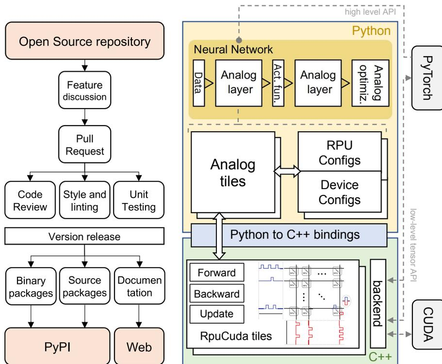
Figure 1: Repository and code structure of the IBM Analog Hardware Acceleration Kit.
