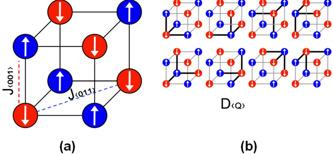
Figure 1: Simplified model of the unit cell (a) with the nearest-neighbor exchange (red dashed line)  $J_{\langle 001 \rangle}$  and the second nearest-neighbor exchange (blue dashed lines)  $J_{\langle 011 \rangle}$ . In (b) eight 4-spin cyclical interactions inside the unit cell (thick dark lines) are shown.
