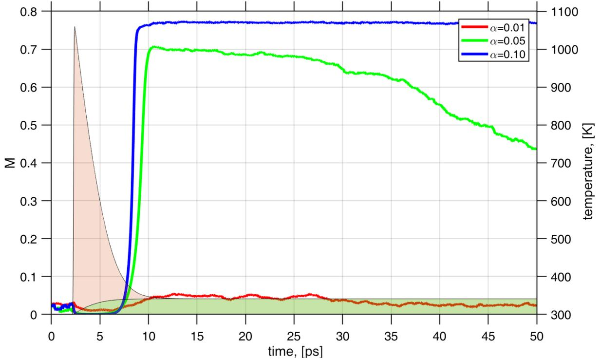
Figure 5: Time dependence of the magnetization for an isotropic particle after laser heating with a 100fs laser pulse for  $\lambda = 0.01$  (red line),  $\lambda = 0.01$  (green line), and  $\lambda = 0.1$  (blue line). The red shaded area defines the electron temperature profile and the green shaded area defines the sublattice temperature.
