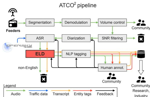
Figure 1: ATCO<sup>2</sup> data flow pipeline. The ELD block is used to filter out non-English speech. The automatically processed data are then annotated and checked by humans. Their feedback is used to adapt particular blocks using active learning approaches.
