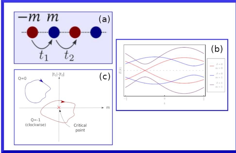
Figure 1: Panel (a): the Rice-Mele lattice. Panel (b): the energy bands for Rice-Mele Hamiltonian for different values of  $m, \delta = |t_1| - |t_2|$  in the 1st Brillouin Zone. The critical point is found at  $m = 0$  and  $\delta = 0$ . Panel (c): the pumped charge  $Q$  after the completion of a full adiabatic cycle is the winding number around the critical point in the parameter space of the Rice-Mele model.
