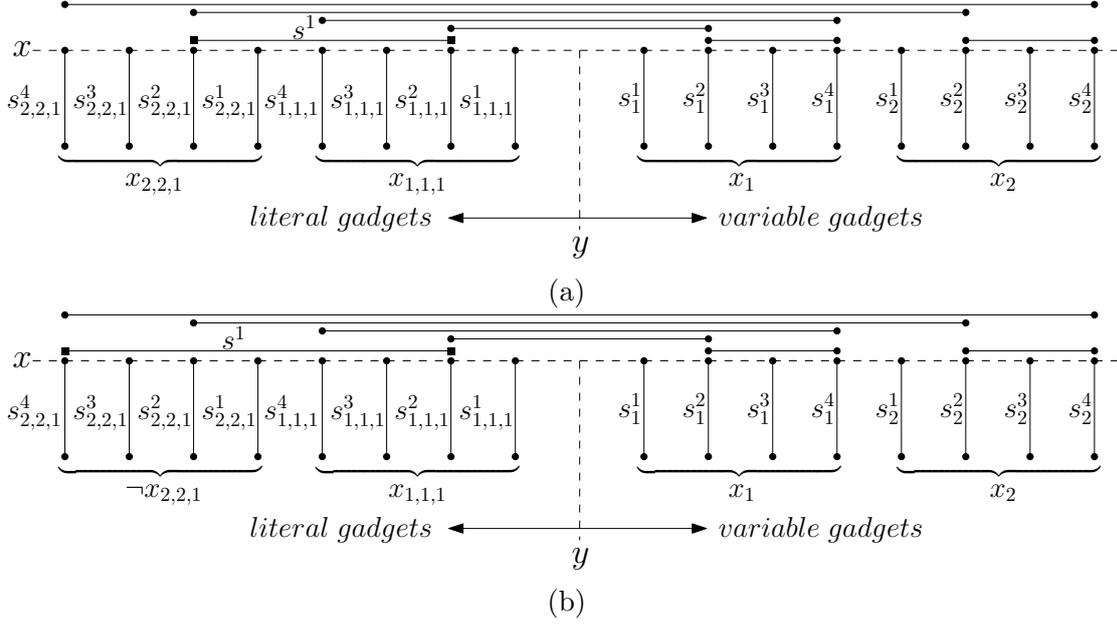
Figure 6: Gadget for the clause (a)  $x_1 \vee x_2$ , and (b)  $x_1 \vee \neg x_2$
