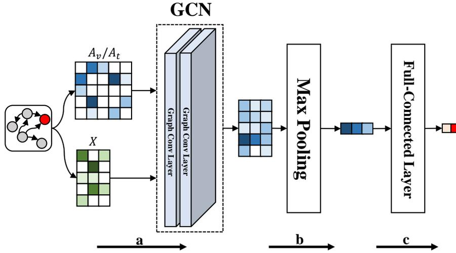
**Fig. 2.** The architecture of I<sup>2</sup>BGNN model. a)  $A_v$  ( $A_t$ ) and  $X$  are captured from subgraph extraction and sent to graph convolution network; b) the max-pooling layer is used to compress the aggregated node representations to obtain the whole graph representation; c) the graph representation is used to predict the subgraph (account) label.
