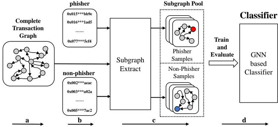
**Fig. 1.** The schematic depiction of our framework. The complete workflow proceeds as follows: a) modeling the transaction network; b) sampling the labeled accounts; c) extracting the subgraphs centered on target accounts; d) training and evaluating using GNNs.
