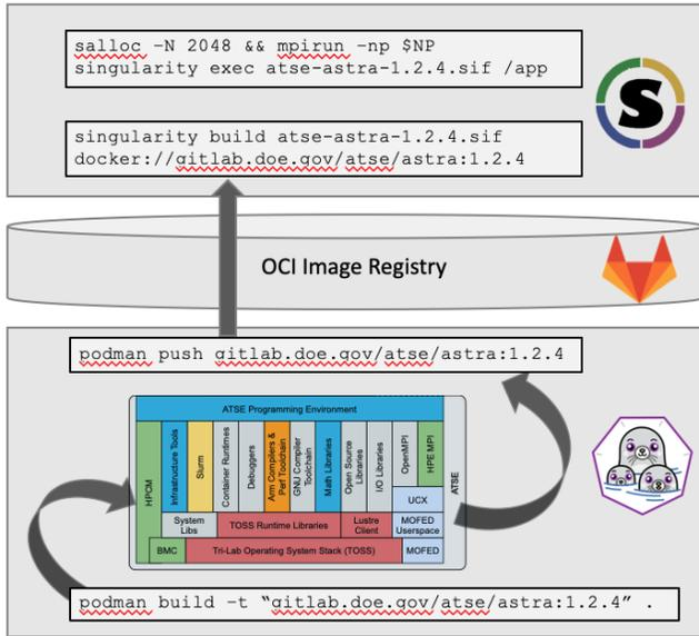
**Figure 6: Container Build Workflow on Astra, with Podman**
