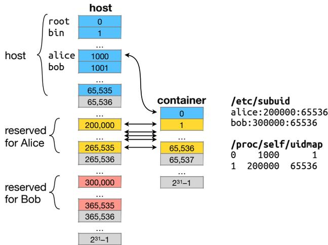
**Figure 1: Typical privileged UID map for container run by Alice. The file `/etc/subuid` configures the user-space helper for host UIDs Alice and Bob may use; `/proc/self/uidmap` is the subsequent kernel mapping.**
