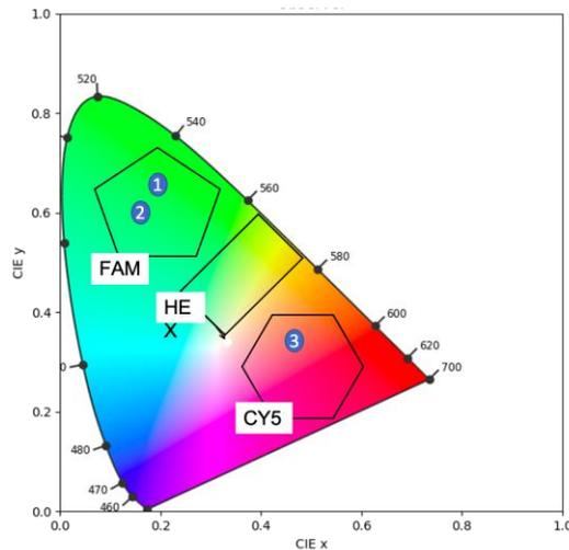
Figure 6 Multiplex detection of Anyplex™II MTB/MDR assay is plotted for Mycobacterium tuberculosis and resistance to Isoniazid (4 mutations in katG)
