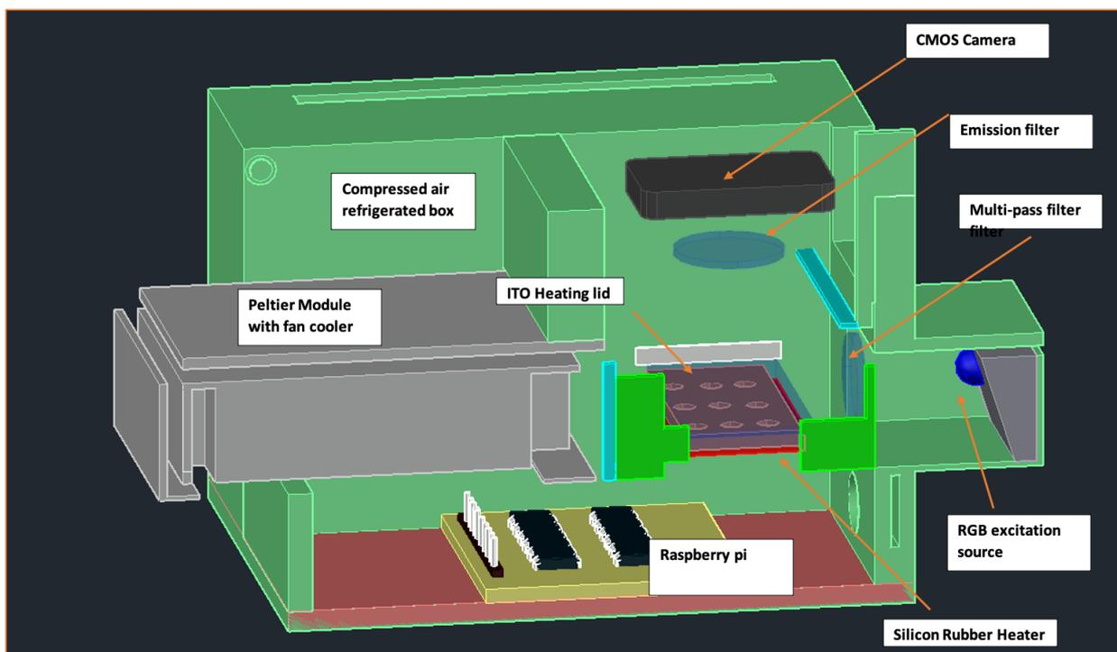
Fig 1. 3D Model render of the proposed device with cross sectional view, it covers all description of the heating and cooling elements as well as optical imaging system of the device
