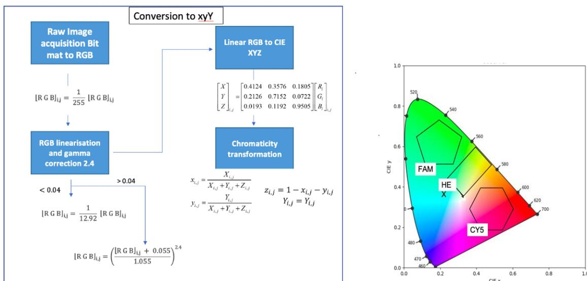
Figure 3. a) Shows the algorithm for image processing as RGB image data set is converted to be represented on a CIE chromaticity diagram [14], b) Die islands are shows as processed in the algorithm
