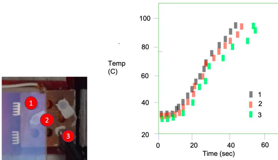
Figure 2. Temperature Characterisation of the copper base is shown to shown as the temperature measured on the dots represented in 2.a) are mapped against time in 2.b). The figure shows isothermal behaviour over the whole testing surface.
