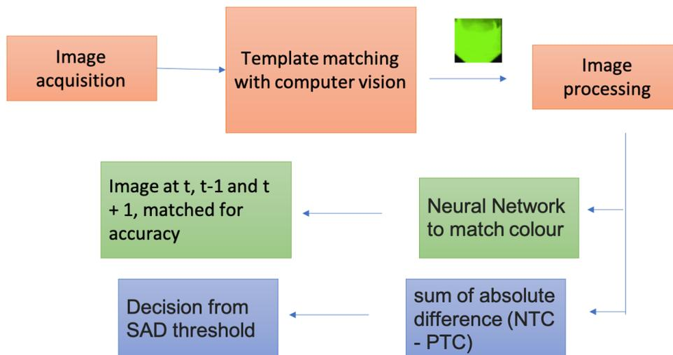
Figure 4 Shows the two methods considered for image acquisition and sensitive detection, data proves that trained neural network method is highly successful
