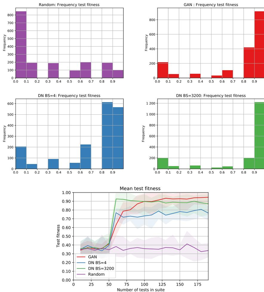
Fig. 3. Test Fitness for Odroid Power  $\geq$  6W
