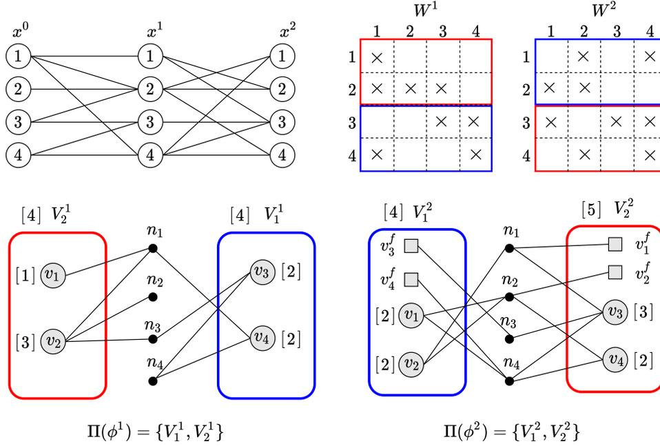
**Figure 3: Top: A 3-layer sparse DNN and the corresponding weight matrices  $W^1$  and  $W^2$ . Bottom: Hypergraphs  $H(\phi^1)$  and  $H(\phi^2)$  built for weight matrices. Partitions  $\Pi(\phi^1)$  and  $\Pi(\phi^2)$  induce a 2-way partitioning on weight matrices.  $[\cdot]$  next to a vertex or a part shows the weight associated with that vertex and part, respectively.**
