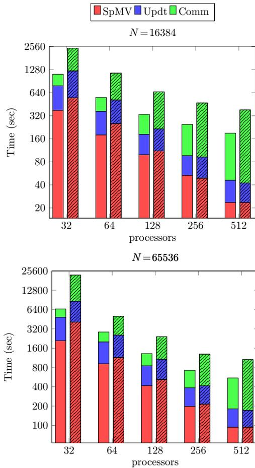
**Figure 5: Breakdown of running time of H-SGD (solid) and SGD (tiled). “SpMV” corresponds to time spent on local sparse matrix-vector multiplications. “Updt” corresponds to the time spent on gradient update operations. “Comm” corresponds time spend for communication operations.**
