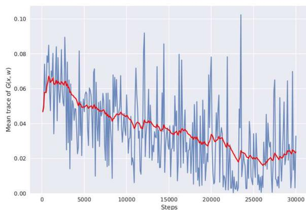
Figure 2. The blue line is the mean trace of  $G(x, w)$  for a batch of images during training. The red line represent the trend of the mean trace obtained through an exponential moving average.
