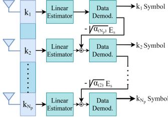
Fig. 2: SSD process on selected receive antennas.
