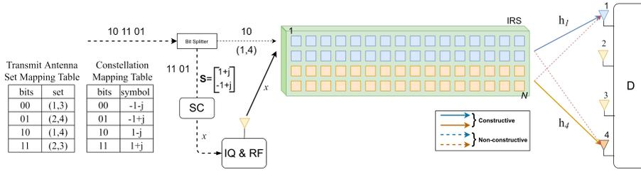
Fig. 1: IRS-assisted communication system with  $N_r = 4$  and  $N_p = 2$ .
