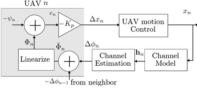
Fig. 3: The closed loop feedback system in UAV  $n$  where  $n \in \{1, \dots, N-1\}$ . The calculations made on the UAV are highlighted in gray. The value  $\Delta\phi_{n-1}$  is obtained from the previous neighbor.
