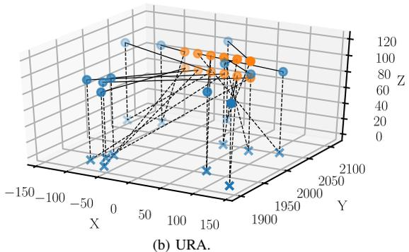
Fig. 6: Blue dots represent the initial positions, orange dots the final positions of the UAVs. The dashes on the ground represent the point of interest. While URA and Cent optimize capacity, URA moves the UAVs significantly far from their points of interest.
