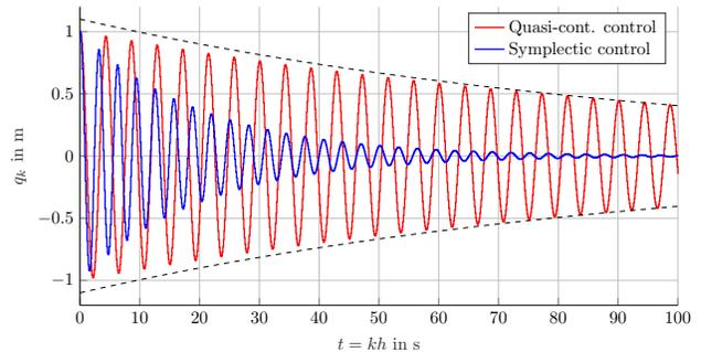
Fig. 2. Initial value responses  $q_k$  with maximum achievable stiffness  $c_{\max}$  for  $h = 0.1$  s (see Fig. 3). Not only is  $c_{\max}$  higher under symplectic control, but also the  $L_2$  norm  $\|q_k\|_h$  is smaller for input signals with identical energy (see Fig. 4).
