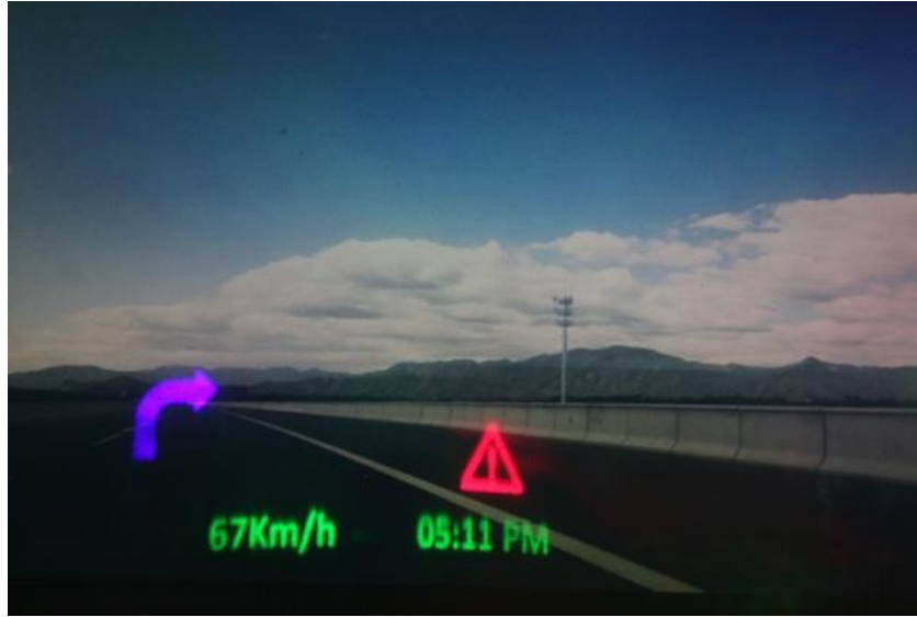
Fig. 8. The AR display effect of the multi-plane holographic HUD system.
