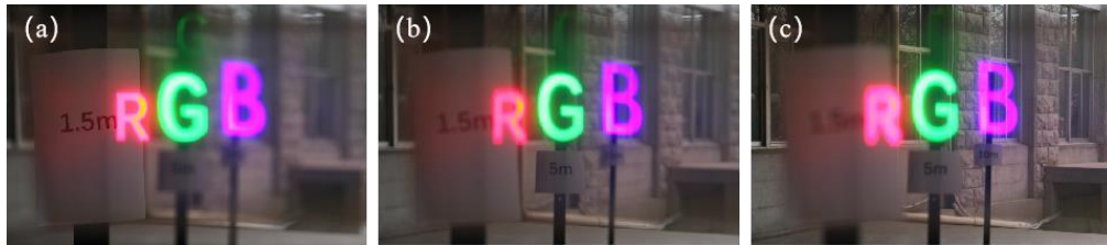
Fig. 7. (a), (b) and (c) are the display effects when the camera focuses on the three letters R, G and B at different distances.
