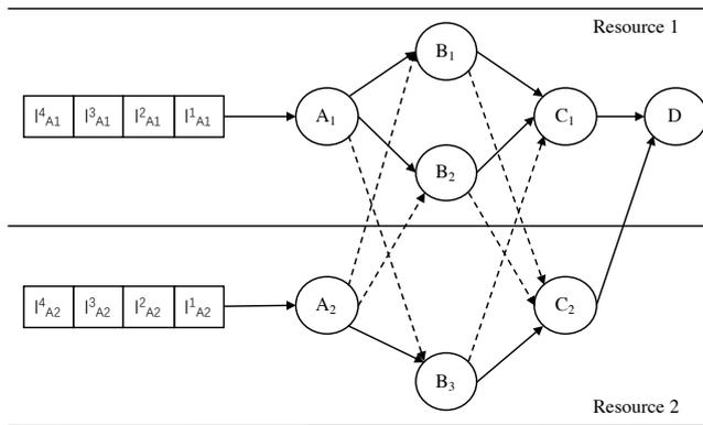
**Fig. 4** Model parallelism. The dashed arrows represent inter-computing resource communication. For each input data point  $I$ , different parts, i.e.,  $I_{A_1}$  and  $I_{A_2}$ , are distributed at different computing resources.
