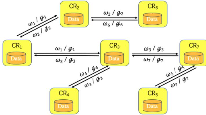
**Fig. 8** The architecture of decentralized aggregation. “CR” represents computer resource.  $\omega$  represents the local parameters, or the weights of the model calculated in each computing resource.  $g$  represents the local gradients in backward propagation in each computing resource. When two computing resources are neighbors, they can communicate with each other.
