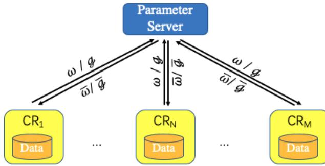
**Fig. 6** The architecture of centralized aggregation. “CR” represents computer resource.  $\omega$  represents the local parameters or the weights of the model calculated in each computing resource.  $g$  represents the local gradients in backward propagation in each computing resource.  $\bar{\omega}$  represents the global model calculated in the parameter server.  $\bar{g}$  represents the global gradients calculated in the parameter server.
