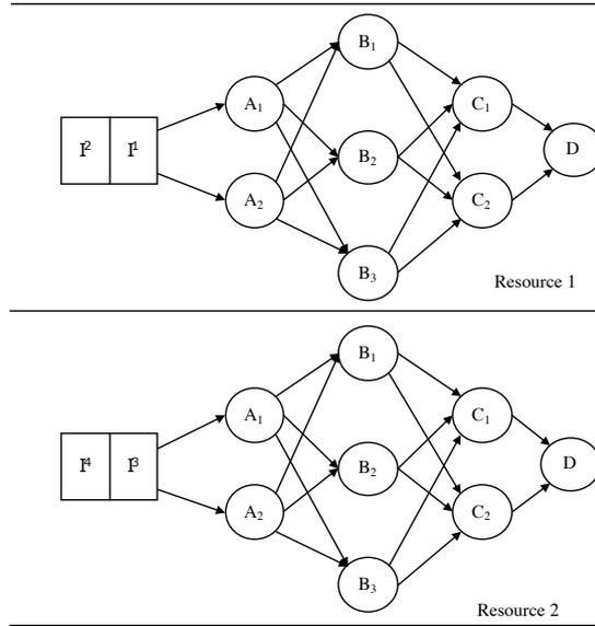
**Fig. 3** Data parallelism. The forward and backward process of  $I^1$  and  $I^2$  is performed in computing resource 1, while that of  $I^3$  and  $I^4$  is performed in computing resource 2 at the same time. Then the model or gradient is transferred to calculate an average model or gradient to be sent to each computing resource for the following training.
