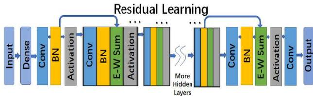
FIG. 1. Schematic diagram for ResNet involving a series of identically-distributed one-dimension convolutional (Conv) layers and batch normalization (BN) layers. At each convolutional layer it has a dilation rate except the first and the last layers. Different from the original convolutional NN scheme, arrows acting on Element-wise sum layers(E-W sum) can preserve the former hidden layer’s information which facilitate the performance of DL.
