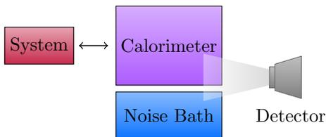
FIG. 1: Schematic representation of the system-calorimeter-noise bath setup. The system and calorimeter interact while the energy of the calorimeter and noise bath is simultaneously measured.
