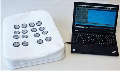
Fig. 1. Multi-channel lung sound recording device.
