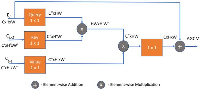
Fig. 3. The overall architecture of AGCM. It takes current encoder features  $E_l$  as Query and concatenates features ( $C_{l-1}$ ) generated from ( $D_{l-1}$ ,  $AGCM_{l-1}$ ,  $SFEM$ ) as Key and Value to perform cross attention.
