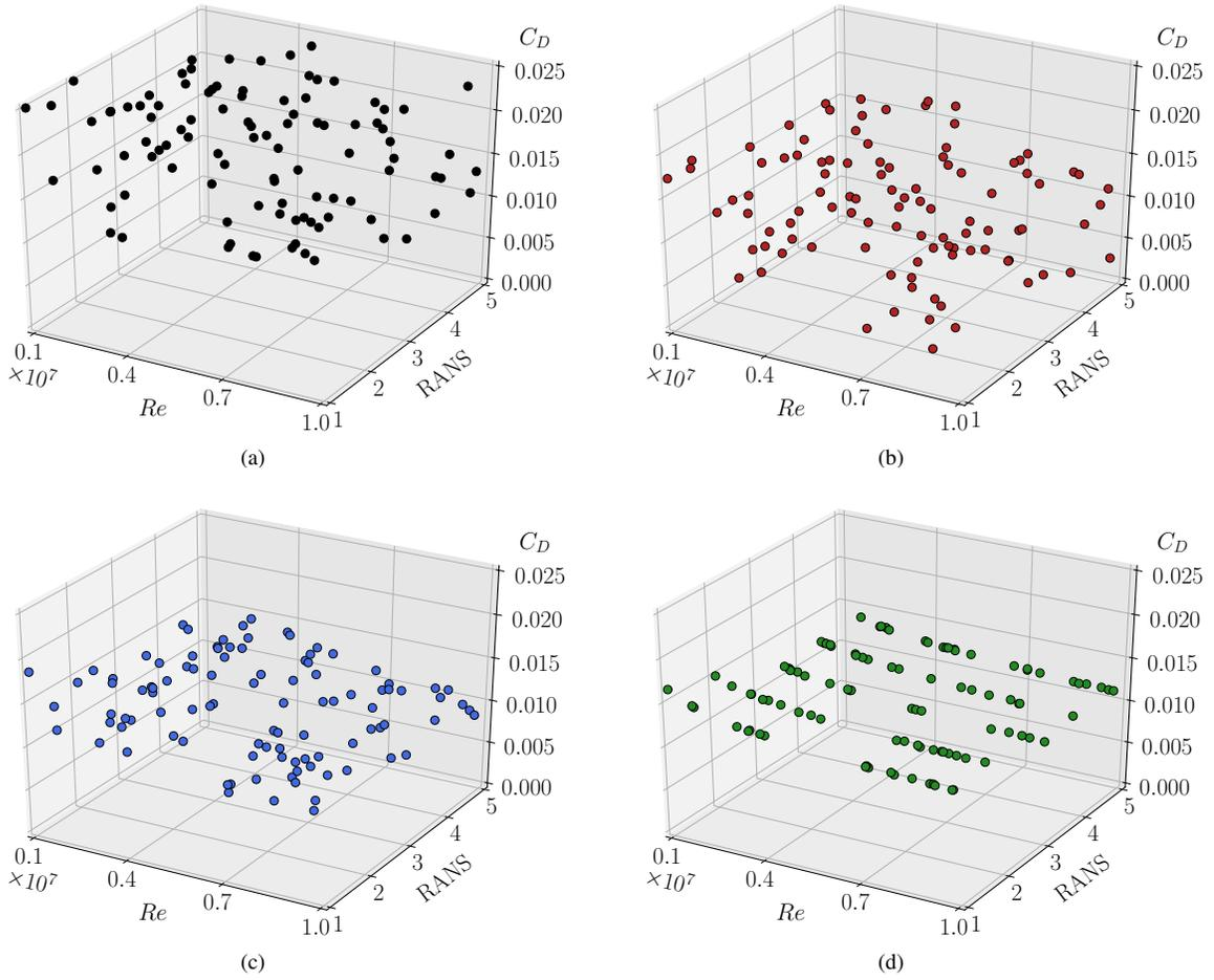
**Fig. 3 Drag coefficient distributions for the parameter space study obtained from the optimized airfoils using the DSP (a) and average/robust [with  $\lambda = 0$  (b),  $\lambda = 10$  (c),  $\lambda = 100$  (d)] design strategies.**
