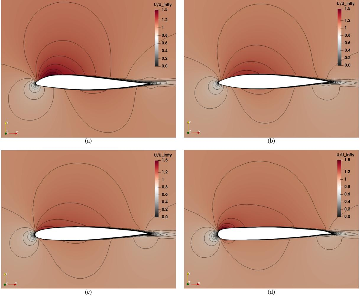
**Fig. 2** Normalized time-averaged velocity fields, i.e.,  $U/U_\infty$ , obtained from the optimized airfoils using the DSP (a) and average/robust [with  $\lambda = 0$  (b),  $\lambda = 10$  (c),  $\lambda = 100$  (d)] design strategies.
