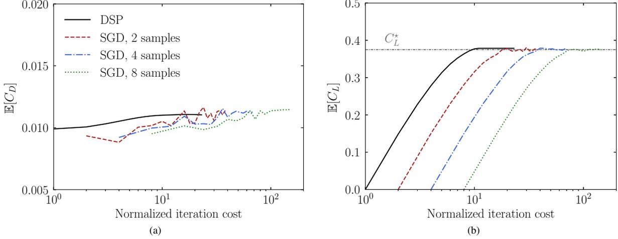
**Fig. 1** Evolution of mean drag (a) and lift (b) coefficients along the optimization iterations expressed in terms of normalized cost for the DSP and average (using  $n = 2, 4, 8$  samples per iteration) design strategies. The horizontal dot-dash line in (b) indicates the target lift coefficient  $C_L^* = 0.375$ .
