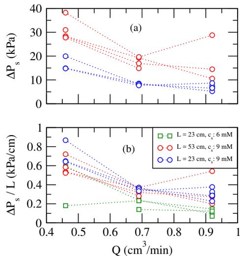
FIG. 3. Variation of (a) saturated pressure drop ( $\Delta P_s$ ) with flow rate in a tube of diameter ( $D = 0.1$  cm) and salt concentration ( $c_s = 9$  mM) for two different tube lengths and (b) Variation of  $\Delta P_s/L$  with flow rate in a tube of diameter ( $D = 0.1$  cm) and two salt concentrations and tube lengths.
