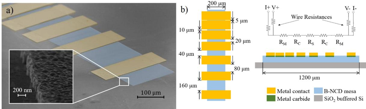
**Figure 3:** (a) false colour tilted SEM of metal contacts on a B-NCD diamond mesa on SiO<sub>2</sub> buffered silicon, with zoomed inset showing the edge profile resulting from the ICP-RIE process. (b) plan (left) and cross section (right) diagrams of the TLM patterns used.
