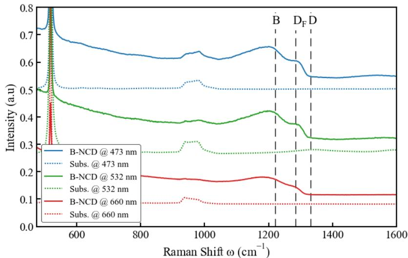
**Figure 1:** Three wavelength Raman shifts of the B-NCD film and substrate (donated “B-NCD” and “Subs.”), where the lack of diamond peak (D) at  $1332 \text{ cm}^{-1}$  and strong peak (B) at  $\sim 1220 \text{ cm}^{-1}$  is indicative of high levels of boron doping.
