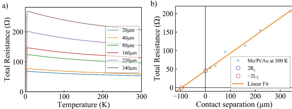
**Figure 4:** (a) example dataset of contact resistances of different contact separations across the temperature range, (b) example linear fit of an isothermal slice through the data (error bars derived from precision of these single resistance measurements are of negligible size).
