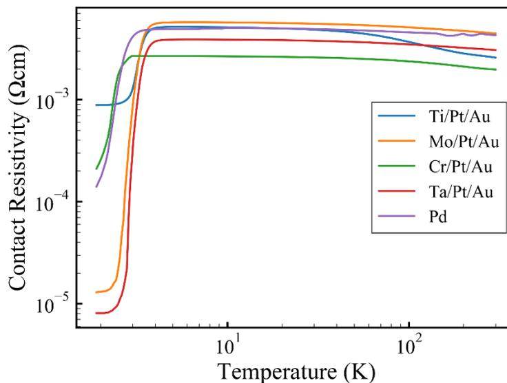
**Figure 5:** Contact resistivity of the various contact schemes scaling with temperature. From 300K to the superconducting transition all the schemes show a slight increase in resistivity, where a significant reduction of the contact resistivity is then observed.
