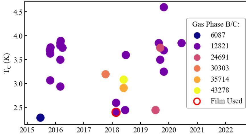
**Figure 2:** The critical temperature of BDD films grown on different dates with various gas phase B/C ratios. The film growths are tuned for different purposes and have various thicknesses but show consistent superconducting performance.
