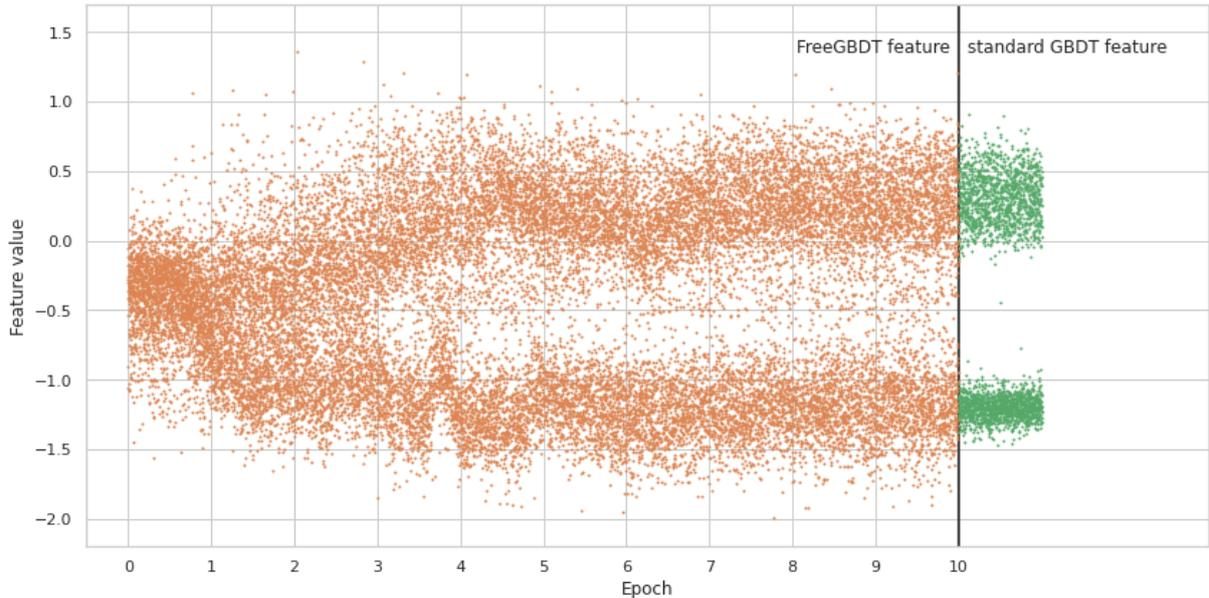
Figure 4: Values of a typical dimension from the 1,024 dimensional vector stored *during* fine-tuning to train a FreeGBDT (left). The same dimension extracted *after* fine-tuning to train a standard GBDT (right).
