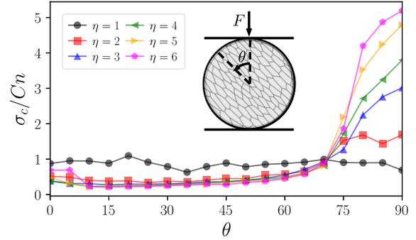
**Figure 2.** Failure strength as a function of the level of inherent anisotropy  $\eta$  and the loading orientation  $\theta$ . In the inset: schematic representation of our loading procedure and the relative loading orientation relative to the rock layering.
