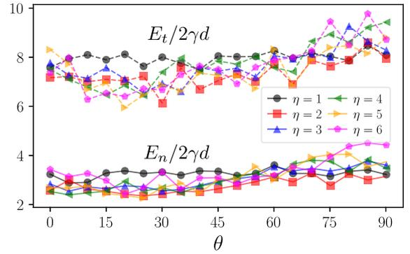
**Figure 5.** Total energy consume at failure in traction and shearing modes as a function of  $\theta$  and different  $\eta$ .
