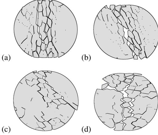
**Figure 3.** Evolution of the failure mechanism as the loading orientation increases (a)  $\theta = 0^\circ$ , (b)  $\theta = 30^\circ$ , (c)  $\theta = 60^\circ$  and (d)  $\theta = 90^\circ$  for the sample with inherent anisotropy  $\eta = 2$ .
