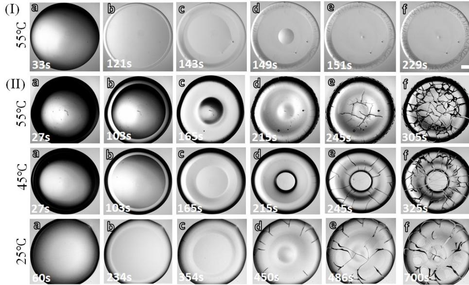
**FIG 3.** Drying evolution of lysozyme droplets: (I) a-f displays  $\phi$  of 1 wt% drying under 55 °C. (II) a-f shows the  $\phi$  of 20 wt% drying at 55, 45, and 25 °C. The timestamps are shown at the left-bottom of each image. The white rectangle represents a scale bar of length 0.2 mm in the top-right.
