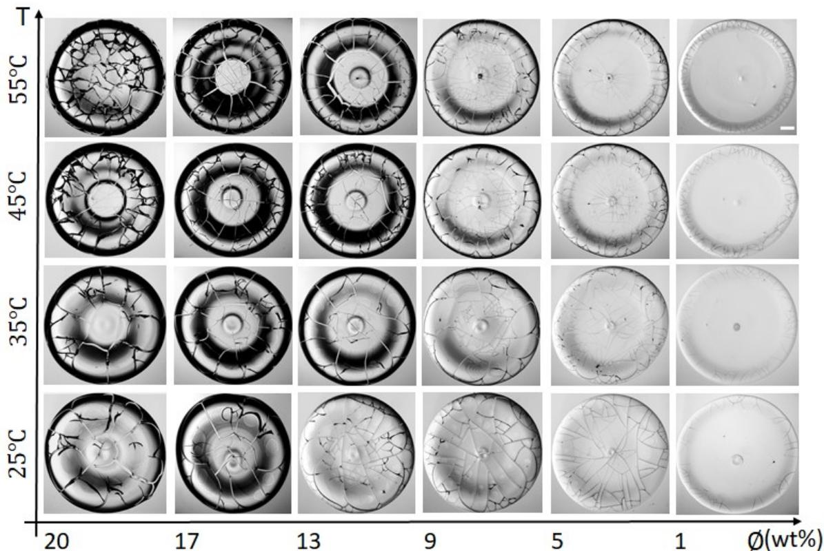
**FIG 1.** Morphology of dried lysozyme droplets captured within 24 hours at various initial concentrations ( $\phi$ ) diluted from 20 to 1 wt% at controlled substrate temperatures ( $T$ ) of 25 to 55  $^{\circ}\text{C}$ . The white rectangle represents a scale bar of length 0.2 mm in the top-right panel 55  $^{\circ}\text{C}$ .
