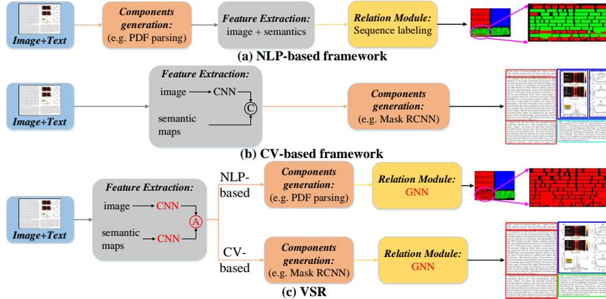
**Fig. 1.** Comparison of multimodal document layout analysis frameworks. VSR supports both NLP-based and CV-based frameworks. © and Ⓐ denote *concatenation* and *adaptive aggregation* fusion strategies. Different colored regions in the prediction results indicate different semantic labels (Paragraph, Figure, Figure Caption, Table Caption).
