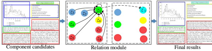
**Fig. 3.** Illustration of relation module. It captures relations between component candidates, and thus improves detection results (remove false Figure prediction, correct Table Caption label and adjust Paragraph coordinates). The colors of semantic labels are: Figure, Paragraph, Figure Caption, Table, Table Caption. Best viewed in color.
