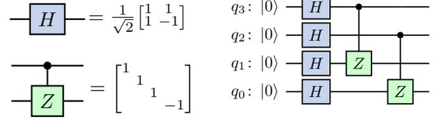
Fig. 1. Quantum gates and quantum circuit  $G$
