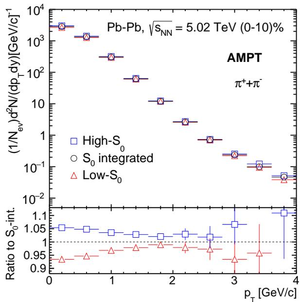
FIG. 2: (Color Online) Top plot:  $p_T$ -spectra for pions in (0-10)% central Pb-Pb collisions for high- $S_0$ ,  $S_0$ -integrated and low- $S_0$  classes. Bottom plot: Ratio of  $p_T$ -spectra for high- $S_0$  and low- $S_0$  events to the  $S_0$ -integrated events.
