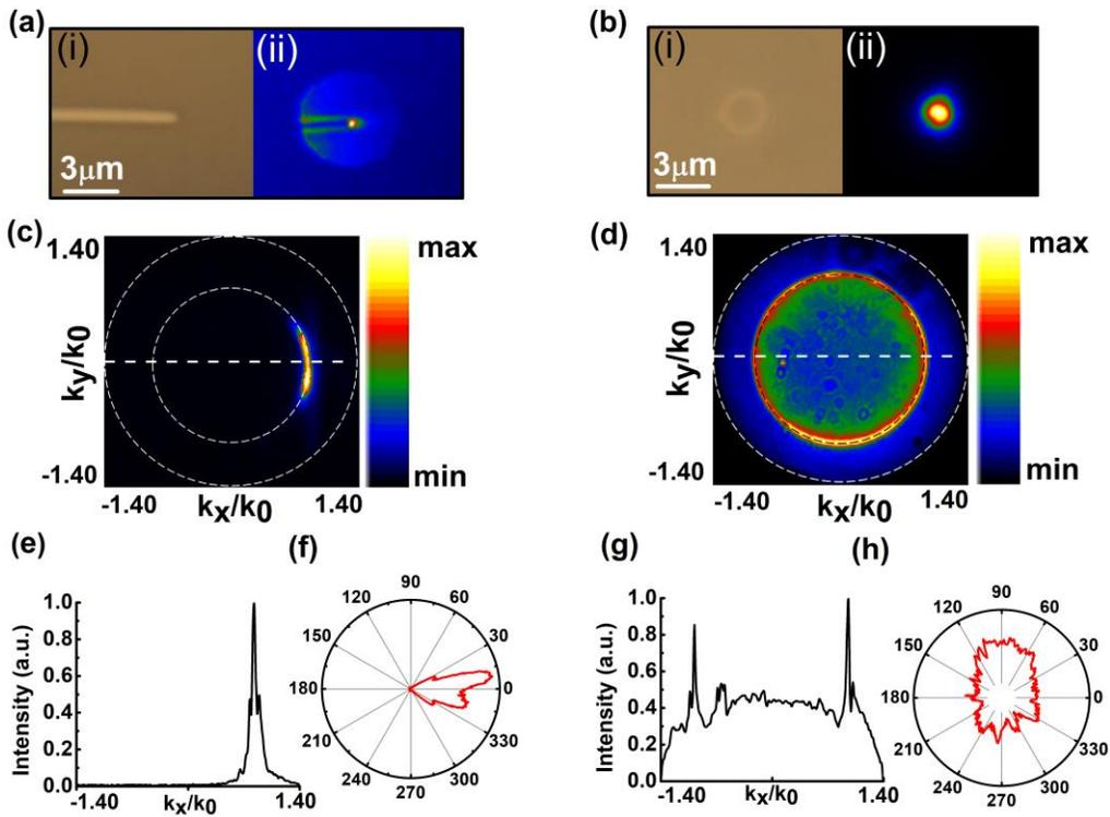
*Fig. 3. Whispering gallery modes wavevector comparison of emission from nanowire end with the emission from isolated microsphere. (a) (i) Bright field (ii) inelastic scattering images of spatially filtered nanowire end. (c) Fourier plane image of the emission collected from distal end of*
