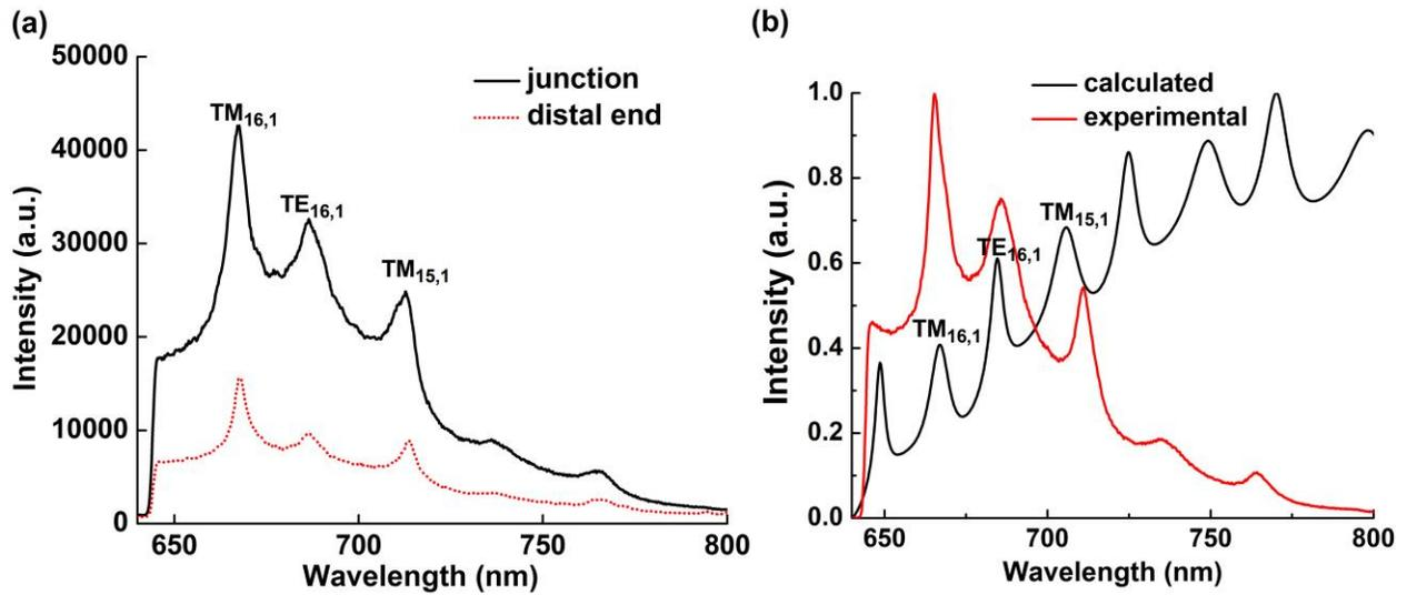
Fig. 2. Spectral signatures of whispering gallery modes. (a) WGMs of a microsphere coupled to nanowire. Black and red curves show the spectral signatures of the emission collected from the AgNW- $\mu$ S junction and nanowire end respectively. (b) WGMs of an isolated microsphere. Red curve shows the experimentally obtained WGMs of an isolated dye coated microsphere placed on a glass substrate. Black curve shows the calculated WGMs of an isolated microsphere in a medium of refractive index 1.
