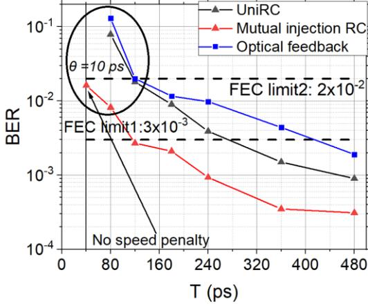
Fig. 6: Comparison between uniRCs and mutual injection RC architectures for 45km of transmission in single mode fiber as a function of  $T$ .  $\theta=20$  ps in all cases, except from those indicated in the circle, where  $\theta=10$  ps.
