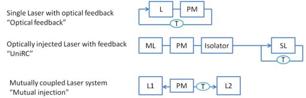
Figure 2: Block diagram of the three different schemes implementing Time-Delayed RC. From top to bottom we see the optical feedback, the unidirectional injection locking combined with optical feedback at the slave and the mutual injection locking architectures.
