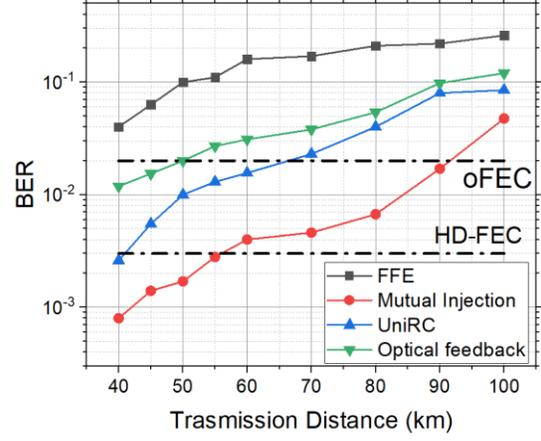
Fig. 7: Comparison between a linear equalizer, uniRCs and mutual injection RC for different transmission distances of the PAM-4 signal. Mutual injection scheme outperforms the other techniques.
