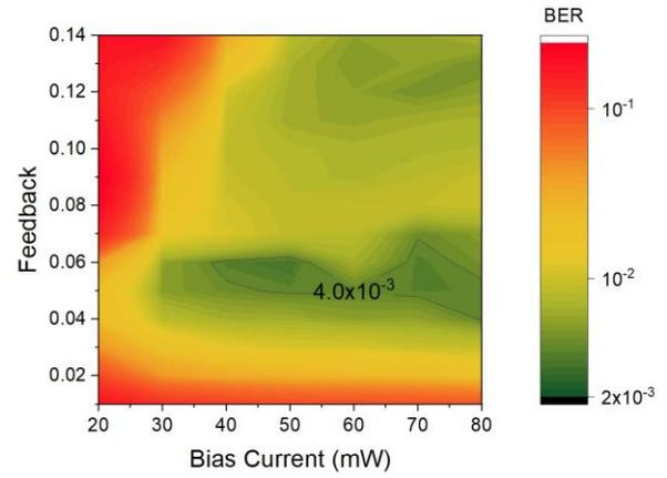
Fig. 5. BER results versus Bias current and Feedback strength for the single laser with phase modulation inside cavity (Optical Feedback). With a delay cavity of 480 ps and 45 km transmission this scheme can provide adequate results for feedback strength around 0.05 and bias current above 30 mW. We choose this best regime for the comparison with the other schemes.
