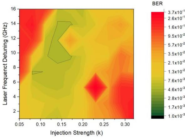
Fig. 3. BER results versus laser frequency detuning  $\Delta f$  and injection parameter  $k$  for 50 km of transmission distance.  $T=240$  ps. The two Lasers are equally biased at 60 mA. Identical results were taken for negative  $\Delta f$ .
