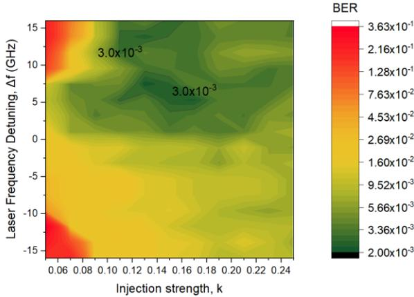
Fig. 4. BER results versus laser frequency detuning  $\Delta f$  and injection parameter  $k$  for 50 km of transmission distance. The two Lasers are unequally biased at 70 mA and 20 mA respectively. BER values slightly below FEC limit of  $3 \times 10^{-3}$  can be obtained.
