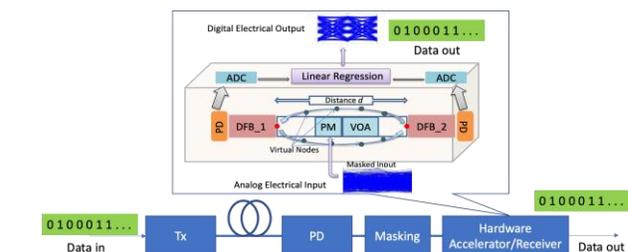
Fig. 1. Fully integrated neuromorphic processor based on mutually coupled Lasers. PM: Phase modulator, VOA: Variable Optical Attenuator, ADC: Analog to Digital Converter, PD: Photodiode, DFB: Distributed Feedback.
