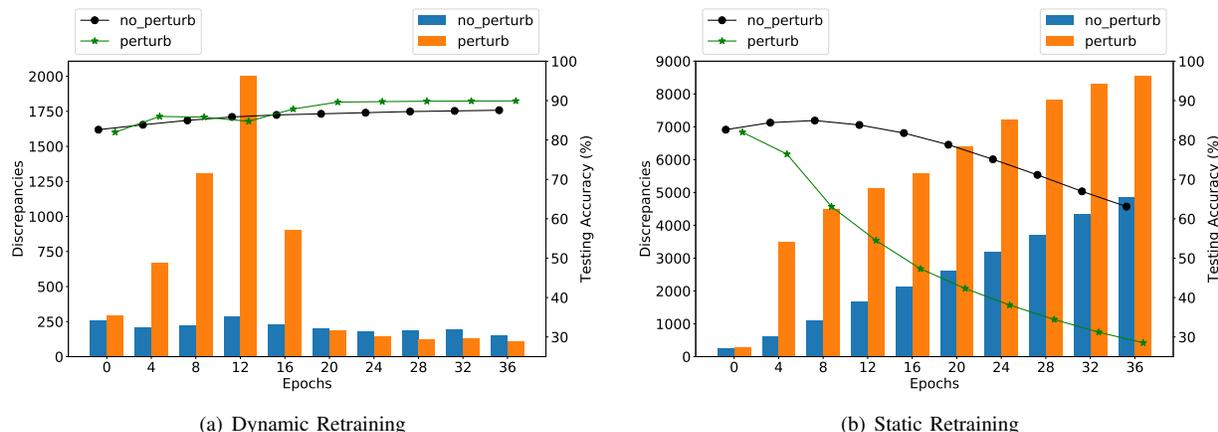
Fig. 5. Accuracy and number of discrepancies of **HDXplore** retrained classifiers on unseen 10000 MNIST images for each epoch of retraining process. We conducted 4 different experiments with the combination of 2 different parameters. (1) Static vs. Dynamic; (2) Perturbation vs. No-perturbation.
