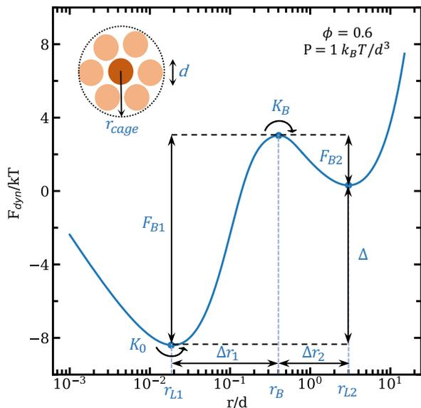
FIG. 1: (Color online) The dynamic free energy of a tagged particle in a hard-sphere fluid of  $\Phi = 0.60$  under compression  $P = 1k_B T/d^3$ . Key length scales and two barriers in the two-state level system are indicated.
