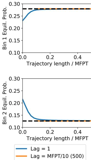
FIG. 2. **MSM equilibrium probability estimates are asymptotically unbiased.** The equilibrium estimator, shown at lag of 1 step ( $\lambda = 1$ , blue) and  $\lambda = 500$  (orange). The black dashed line is the exact reference value, computed from the microscopic matrix. Because the energy landscape is symmetric, only states (‘bins’) in the left half are shown. We assumed a non-informative uniform initial distribution of weights  $w_i(0) = 1/42$ .
