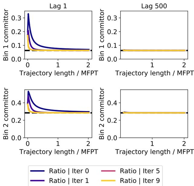
FIG. 7. **Iterative reweighting accelerates committor convergence** Initial committor estimates (dark blue lines) and subsequent iterations (dark purple to orange lines), and reference value (dashed black line). Estimates employ the ratio estimator (23) applied to stationary solutions of the ssMSM and MSM at the trajectory lengths indicated. We assumed a non-informative uniform initial distribution of weights  $w_i(0) = 1/42$ .
