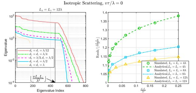
Figure 4: Eigenvalues of  $\mathbf{R}(\tau = 0)$  in non-increasing order for various  $d_x$  and  $d_z$  with  $L_x = L_z = 12\lambda$  (left), and ratios of rank of  $\mathbf{R}(\tau = 0)$  to  $\lfloor \frac{\pi L_x L_z}{\lambda^2} \rfloor$  versus  $\frac{d_x d_z}{\lambda^2}$  for various  $L_x$  and  $L_z$  (right).
