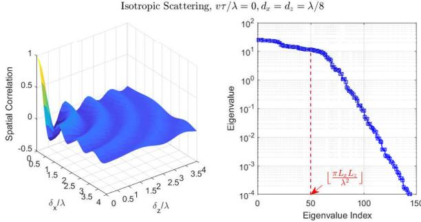
Figure 2: Spatial correlation among RIS elements (left) and eigenvalues of  $\mathbf{R}(\tau = 0)$  in non-increasing order (right) under isotropic scattering, with  $L_x = L_z = 4\lambda$  and  $d_x = d_z = \lambda/8$ .
