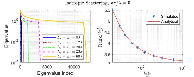
Figure 3: Eigenvalues of  $\mathbf{R}(\tau = 0)$  in non-increasing order for various  $L_x$  and  $L_z$  (left), and ratios of rank of  $\mathbf{R}(\tau = 0)$  to  $\frac{L_x L_z}{\lambda^2}$  versus  $\frac{L_x L_z}{\lambda^2}$  (right), with  $L_x = L_z$  and  $d_x = d_z = \lambda/2$ .
