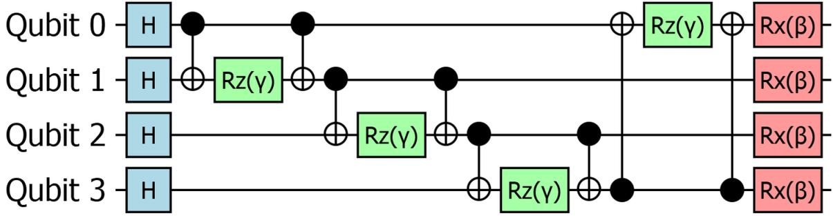
Figure 3: QAOA circuit with  $p = 1$ . H(adamard) gates are applied to all qubits. Then a sequence of controlled z-rotations is performed. The qubits which interact via these controlled rotations is determined by the input graph, shown in Figure 1a. A controlled-z rotation is performed for each edge in the graph. Finally, x-rotations are performed on all qubits. Classical parameters  $\gamma$  and  $\beta$  determine the rotation angles.
