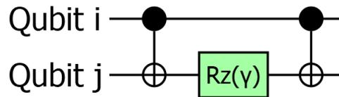
Figure 2: A controlled phase operation between qubit  $i$  and qubit  $j$ . Two CNOT gates and a single-qubit z-rotation is used. The angle of the z-rotation is set by  $\gamma$ , which is a classical parameter.
