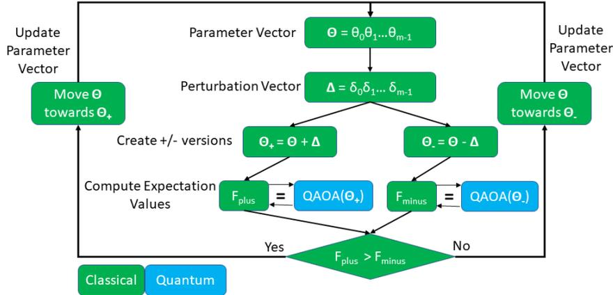
Figure 4: The process of using SPSA to train QAOA. Green blocks are performed on the classical computer, Blue blocks are performed on the quantum computer
