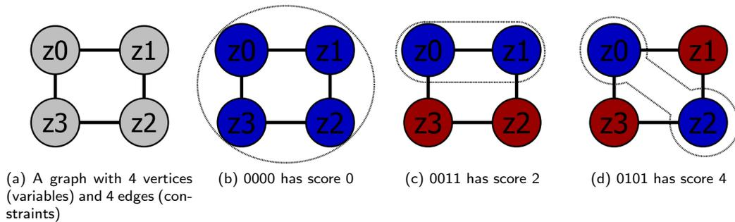
Figure 1: Input to max-cut can be represented by a graph where vertices are variables and edges are constraints. The problem can then be considered a graph coloring, where there are two colors (eg Blue=0, Red=1) and edges should connect vertices of different colors. The number of edges that cross color boundaries (“cut” the set boundaries) represents the score of the coloring.
