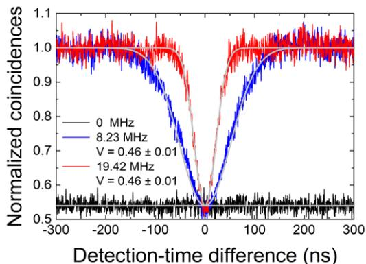
Fig. 2. Normalized coincidences as a function of the detection-time difference between the two single-photon detectors. The Hong-Ou-Mandel-type two-photon interference fringes are measured for three different frequency noises applied to the phase modulator (see text for details).
