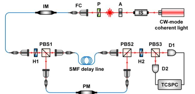
Fig. 1. Experimental setup to observe the two-photon interference of two phase-randomized weak coherent pulses. IS: optical isolator, A: attenuator, P: linear polarizer, FC: single-mode fiber coupler, IM: intensity modulator, H: half-wave plate, PBS: polarizing beam-splitter, PM: phase modulator, D: single-photon detector, TCSPC: time-correlated single-photon counter.
