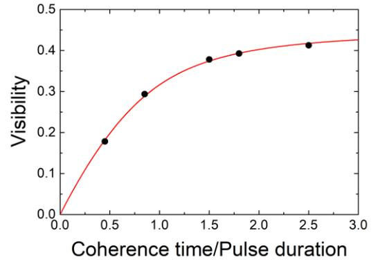
Fig. 4. Two-photon interference fringe visibility as a function of the ratio of the mutual coherence time to the pulse duration.
