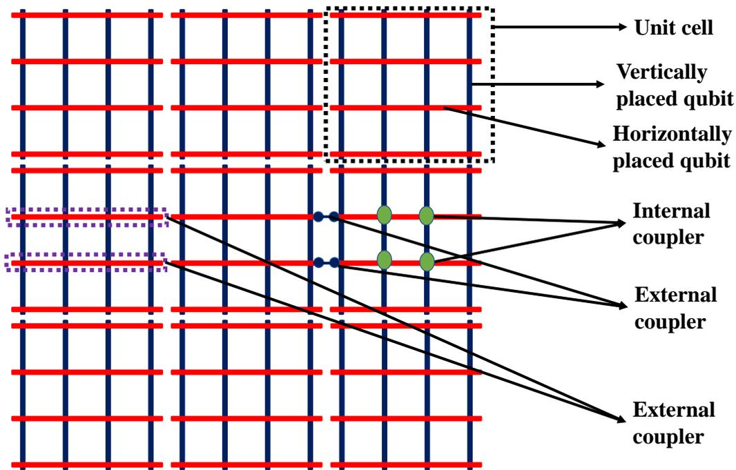
Fig. 5 Architecture of D-Wave's QPU layout
