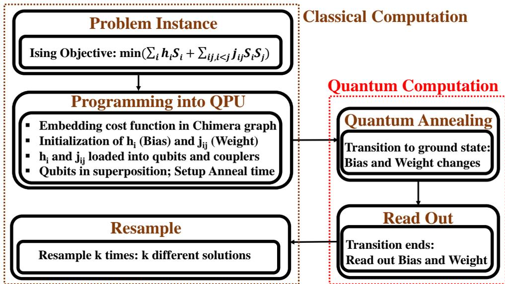
Fig. 4 Overview of the steps required for computation using D-Wave's QPU [31]
