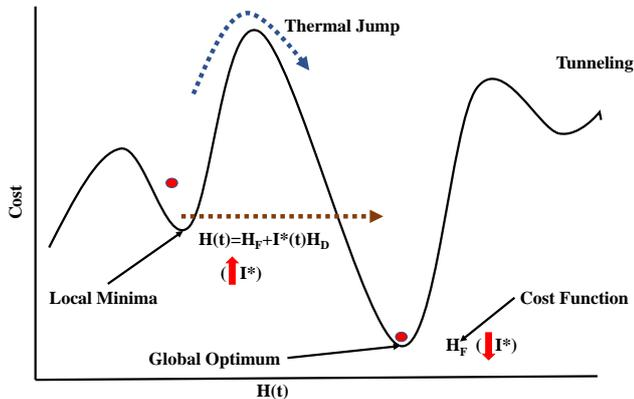
**Fig. 2** Solution landscape of a cost function represented by a time-dependent Hamiltonian. High values of the transverse field coefficient drives tunneling phenomenon in order to escape local minima and move towards the optimal solution.
