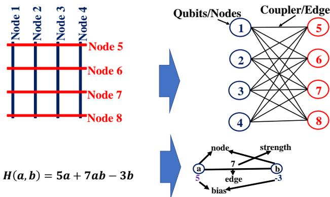
Fig. 6 Graphical representation of a two-variable objective function
