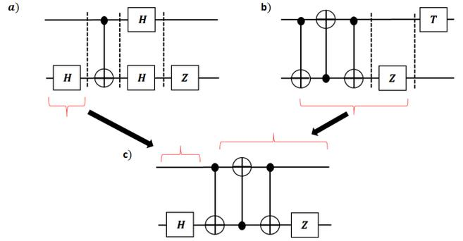
FIG. 4. Example of a crossover involving the leader circuit *a* and the interacting circuit *b*. Notice that although the second and the third blocks in *b* together just add one depth to its circuit, in our approach they are considered two distinct blocks. The new individual *c* is constructed out one block coming from the leader (*H* block) and two from the interacting individual (the *Swap* and *Z* blocks).
