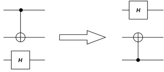
FIG. 6. Controlled block mutation: random shuffling method.
