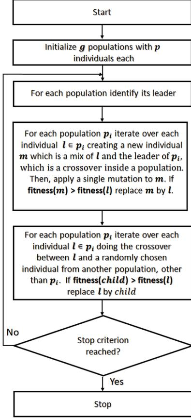
FIG. 3. Fluxogram of the Island model genetic algorithm.
