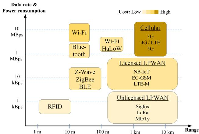
Fig. 5: Wireless communication technologies in IoT [22] [23].
