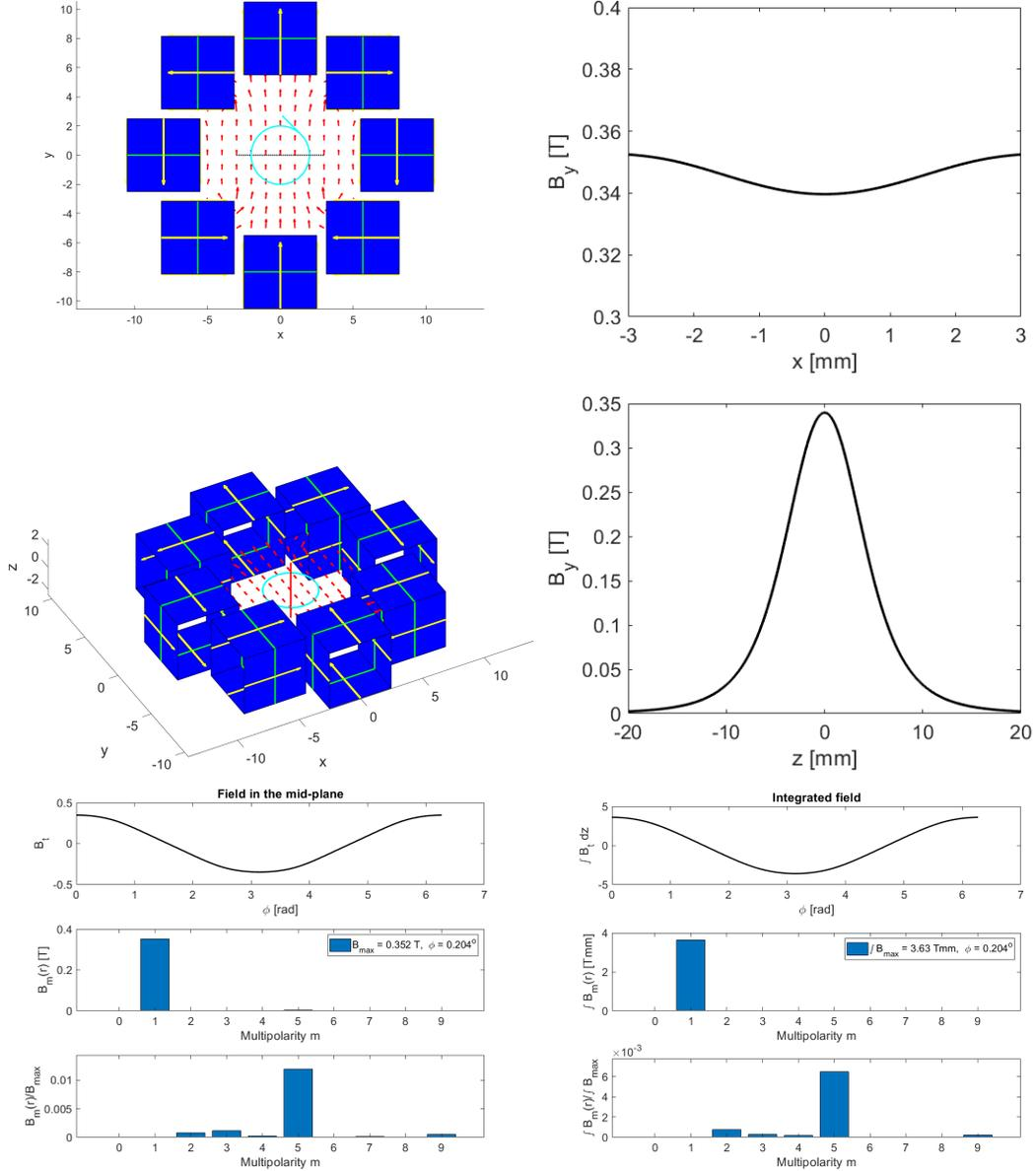
Figure 3: The geometry of a permanent magnet solenoid (top left) and the vertical field in the midplane in the  $x$ -direction (top right). A 3D rendition of the magnet (middle left) and the field along the  $z$ -axis (middle right). The bottom left shows the field along the circle shown in cyan and the multipole coefficients (absolute and relative) in the midplane. The bottom right shows the corresponding integrated values.
